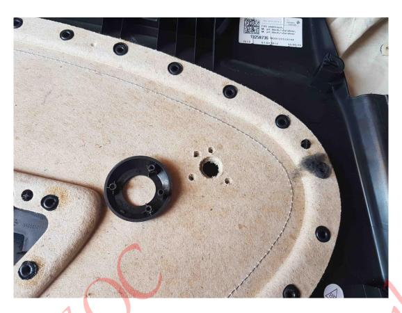
Using 3 x 5mm long screws with penny washers, attach the plastic trim. Do not over tighten the screws as you might break the plastic tabs. I used screws, as that's what I had in my garage.
