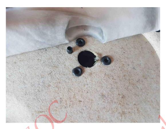
Carefully cut or drill the top of the plastic welds off to remove the trim from the door card.
